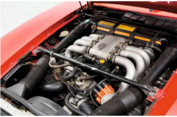
The V8 powering Porsche's big GT grew from 4474 to 5399cc during the 928's 18-year lifetime. Cambelt interval is 60,000 miles
